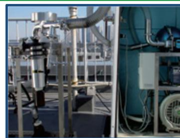
High-Volume Simultaneous Sampler for Fine and Coarse Particles
