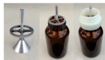
Development of an Attachment to Improve the Collection Efficiency of PM
