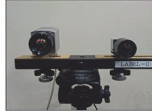
RGB Camera : Point Gray Flea3 IR Camera : Optris PI640
